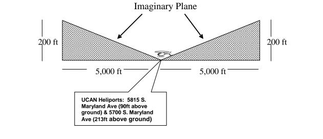
It is the responsibility of the contractor to make provisions for any difference in height elevations of the crane location in relation to the location of the UCAN heliport, when necessary.
