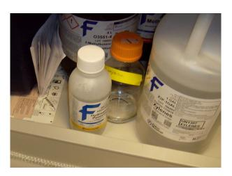
Flammables, like the xylene and 2-methylbutane / isopentane, are liquids that burn easily. They should be kept in a flammables cabinet.
