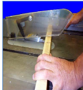
Self-adjusting guard for table saw blade
