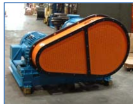
Guard enclosing power transmission apparatus
